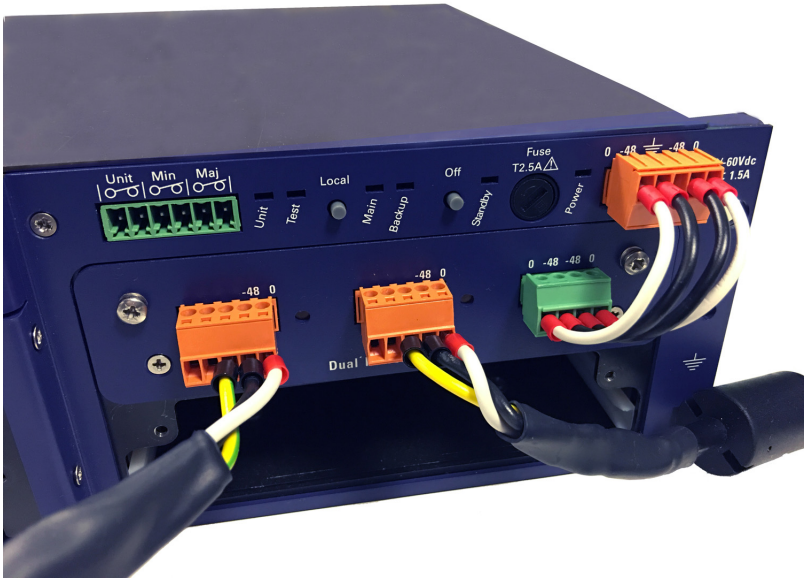
Figure 19 Wiring for Dual power feed
