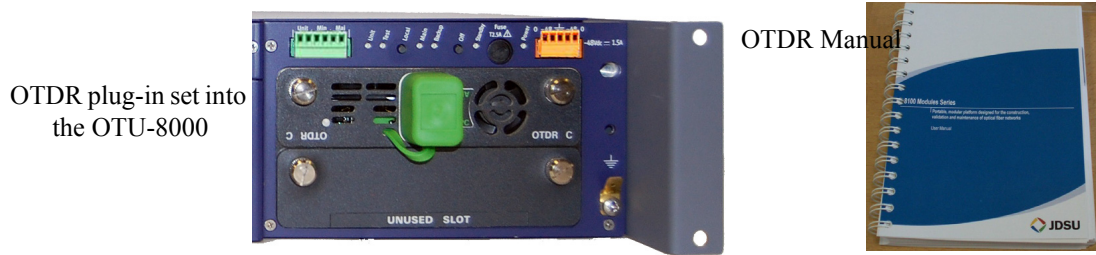
Figure 11 OTDR Module mounted + User Manual
