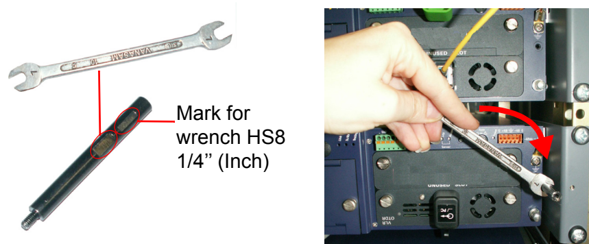
Figure 16 Spacer onto the OTU-8000
